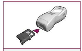
When prompted by the analyser screen, insert the test cartridge.
