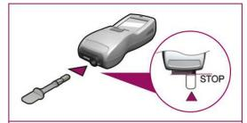
Insert the **collection device** into the **test cartridge** (in the analyser).
